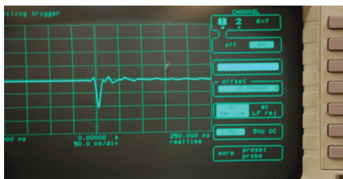
Figure 3 – First discharge pulse that occurs as shown in Figure 1 b)
