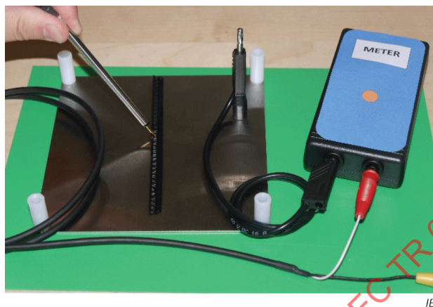
Figure 5 – Single point probe test method set-up
