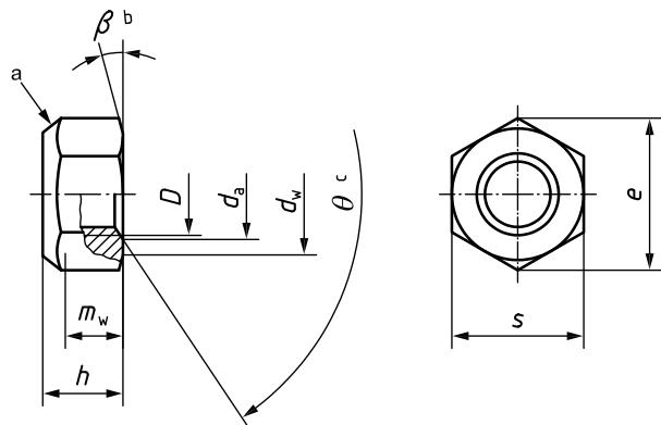
a Prevailing torque element; shape at the discretion of the manufacturer.
