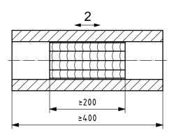
b) Axial overlay welding — Internal
