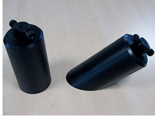
Figure C.1 — Measurement sensor attachments, 90° and 45°
