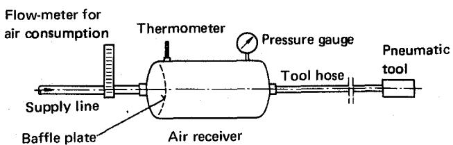
The receiver shall have a cross-section,  $A$  m<sup>2</sup>, perpendicular to the direction of the air stream of at least
