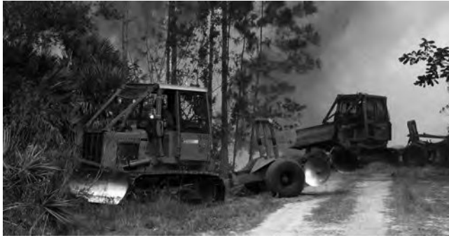
FIGURE A.20.1.3.2(3)(b) Tractor Plows Being Used in Suitable Terrain to Build Firelines. (Courtesy of Florida Division of Forestry)
