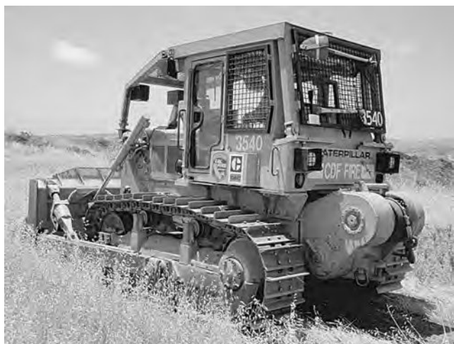
FIGURE A.20.1.3.2(3)(a) A Dozer Equipped with Protective Canopy, Lights, Brush Guards, and a Winch.
