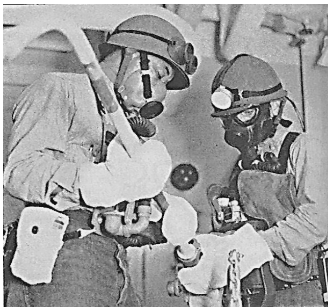
FIGURE 8.3.3.1(b) Navy All-Purpose Nozzle with Adapter Being Installed.
