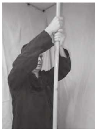
FIGURE 8.26.5.4(a) Position of Test Subject Body, Arms, and Hands with Respect to Pole. (Courtesy of Intertek Testing Services.)
