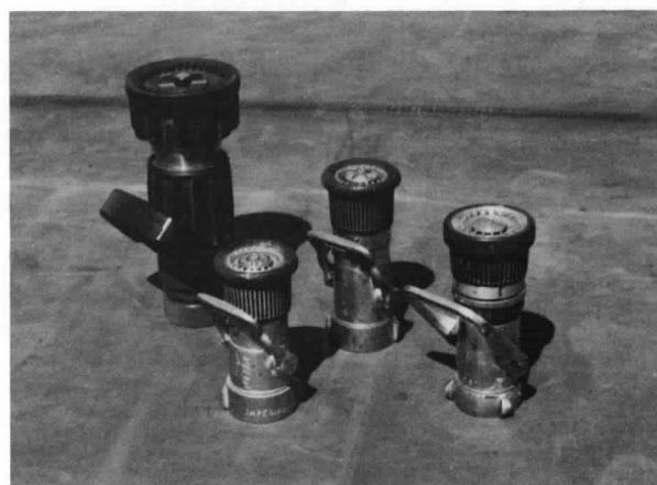
Figure 13-7 Photo shows a variety of typical spray nozzles currently used by structural fire departments. All have the feature of adjustable spray patterns and straight stream settings. Some also have variable flow settings. Most fire chiefs agree that a nozzle setting of 30 degrees provides the best pattern for fighting flammable liquid fires with either water, AFFF, or FFFP solutions.
