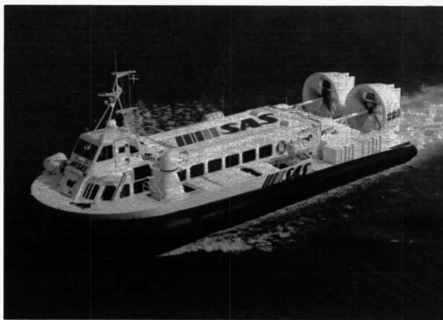
Figure A-3-17 The "Winchester" Class Hovercraft (built by the British Hovercraft Corporation), which is in service at the Auckland International Airport in New Zealand. It is utilized to protect aircraft operations that are largely over the Manukau Harbor that borders the airport. The primary mission is rescue of occupants in event of an accident in the harbor or mudflats (which exist at low tide).
