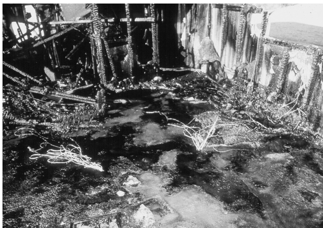
FIGURE 6.17.8.2.3(a) Irregular Burn Patterns on a Floor of a Room Burned in a Test Fire in Which No Ignitable Liquids Were Used.
