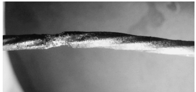
FIGURE 8.10.6.2.1(a) Stranded Copper Conductor in Which Melting by Fire Caused the Strands to be Fused Together.
