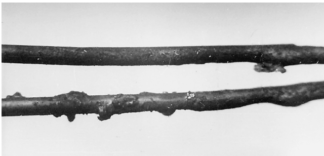
FIGURE 8.10.6.2(a) Copper Conductors Fire-Heated to the Melting Temperature, Showing Regions of Flow of Copper, Blistering, and Surface Distortion.
