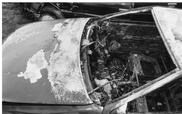
FIGURE 25.8.1.1(c) Radial Burn Pattern Produced by a Passenger Compartment Fire.
