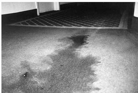
FIGURE 6.17.8.2.3(b) Irregularly Shaped Pattern on Floor Carpeting Resulting from Poured Ignitable Liquid; Burned Match Can be Seen at Lower Left.
