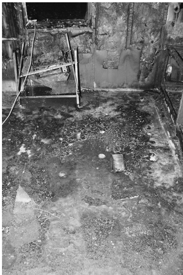
FIGURE 6.17.8.2.5(b) Fire Patterns on Linoleum Floor Resulting from Fully Developed (Post-Flashover) Fire in Full-scale Test Burn of Residential Structure; No Ignitable Liquids Were Present.
