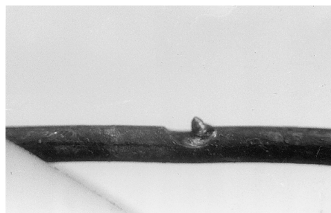
FIGURE 8.10.2 A Solid Copper Conductor Notched by a Short Circuit.
