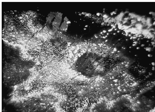
FIGURE 6.17.8.3 Doughnut-Shaped Fire Pattern on a Carpeted Floor.
