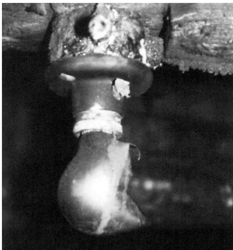
FIGURE 6.20.1 A Typical “Pulled” Bulb Showing that the Heating Was from the Right Side.
