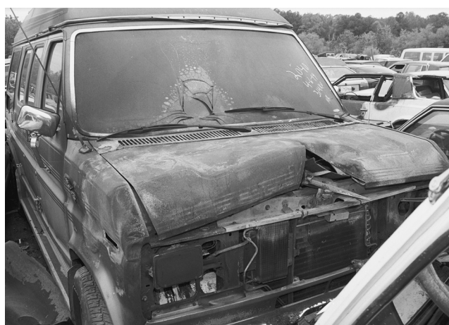
FIGURE 25.8.1.2(a) Incipient Windshield Failure Caused by an Engine Compartment Fire.
