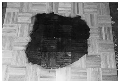
FIGURE 6.17.8.2.3(c) “Pool-Shaped” Burn Pattern Produced by a Cardboard Box Burning on an Oak Parquet Floor.
