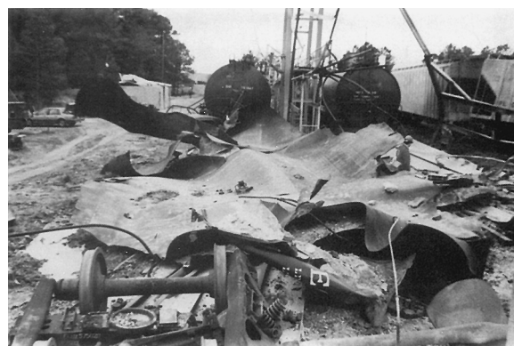
FIGURE 21.2.2.3 A Railroad Tank Car of Butadiene that Suffered a BLEVE as a Result of Heating Created by an Internal Chemical Reaction.
