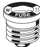
FIGURE 8.6.2.1.1(a) A Typical, Edison-Based Nonrenewable Fuse, Single Element, for Replacement Purposes Only.
