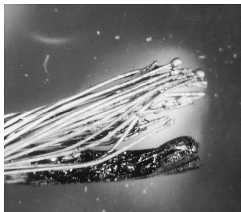
FIGURE 8.10.2.2 Stranded Copper Lamp Cord That Was Severed by a Short Circuit.
