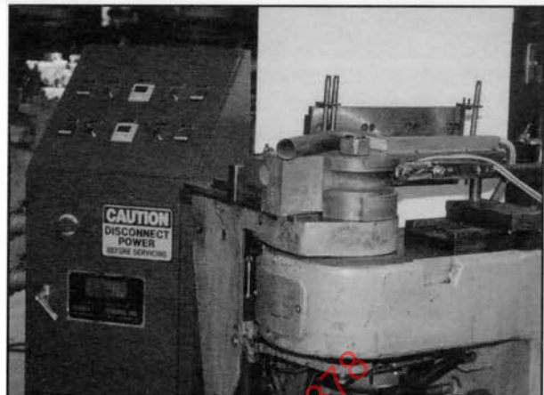
Heated tool set for thin wall titanium aerospace application. In-house test bending included pressure die assist. High-temp lube complete with control cabinet and enough electrical input to dim the lights of Denver.
