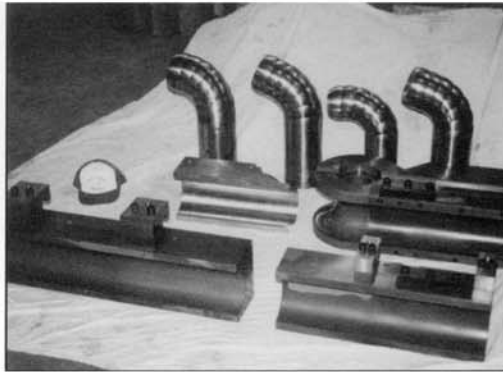
5 piece tool set aerospace application. 5.0 OD x 1 x D (5.0 CLR) captive lip, double rotation, close pitch aluminum bronze mandrels (3) and wiper die. 120° with wiper die clearance and horizontal location and lock of clamp die to clamp insert.
